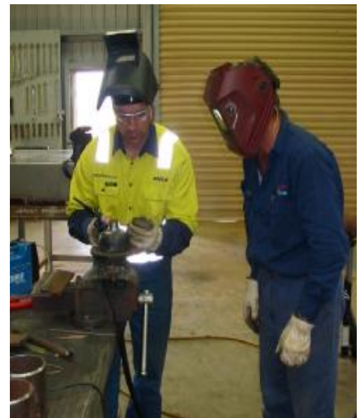
Damien Vickers from Australian Welding Solutions providing some Coaching on how to set a full penetration threadolet onto an end cap of a pressure component
